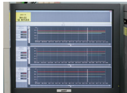
ACTMoS monitoring screen. The vertical white line indicates current data. The data shown on the left side of the white line are analog values previously obtained at registered points, while those on the right of the line indicate predicted values.
