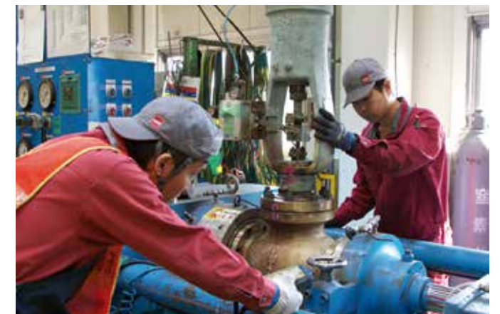
To ensure quality, engineers use specialized test equipment to check a variety of characteristics of repaired valves, including tests of pressure, airtightness, leakage, and operation.
