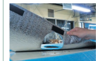
Reflow air heater with insulation
