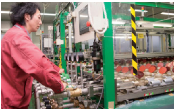
Piston Prover, automatic water meter inspection equipment
