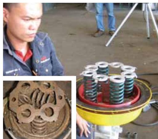
The valve maintenance center in Rayong cleaned 200 water-damaged valves.
