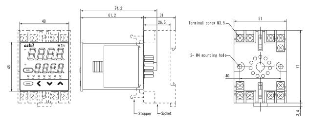
Put the socket stoppers in the upper and lower holes of the main body and secure the socket firmly.
