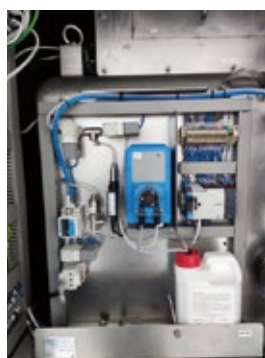
Azbil Telstar's ionHP+ is installed in the isolator and sterilizes the interior of the housing using a hydrogen peroxide solution after completion of the process in the isolator.
