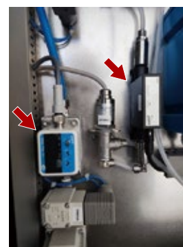
Right: The micro flow rate liquid flowmeter (model F7M), which uses a thermal principle to measure out a micro flow of 20 ml/min of the hydrogen peroxide solution.
