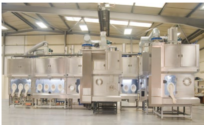
An isolator offered by Azbil Telstar. This piece of equipment ensures the safety of operators by providing an isolation unit where harmful and toxic substances can be processed.
