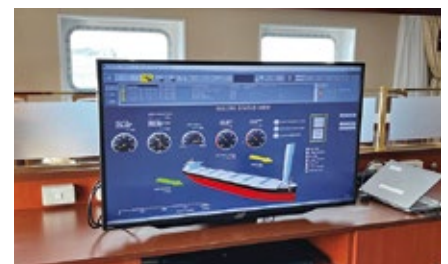
A large monitor installed in the officers’ mess, a cafeteria and conversation space on board. The status of the hard sail controlled by Harmonas-DEO is displayed, and guests who visit the room can check the status of the hard sail in the same way as in the pilot house.
