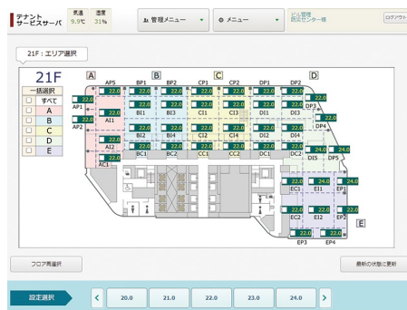
A tenant service screen showing the floor’s air conditioning zones and temperature measurement points.
