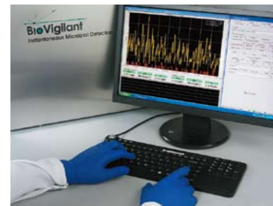
The IMD-A system automatically detects airborne microbes instantaneously and (bacteria and fungi) in real-time.
