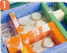
Production of mold Silicon is poured over actual food. The food is removed after the silicon hardens. (Parts of sweets shown in the photo) Vinyl resin is poured into the mold.
