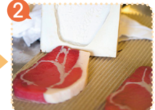
Molding Vinyl resin is heated and hardens in the oven. Pink and white vinyl resins are combined to express the texture of raw meat.
