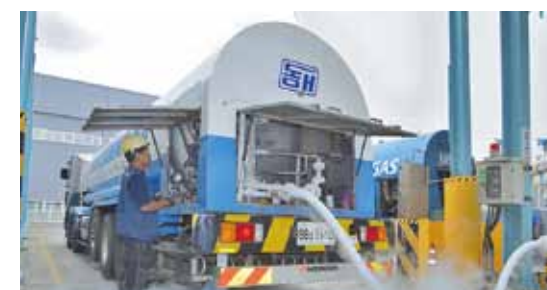
Some of the industrial gases produced at the Ulsan Plant are supplied to the petrochemical complexes of DIG's customers via pipelines, and some are liquefied at ultralow temperatures and delivered by tanker trucks.
