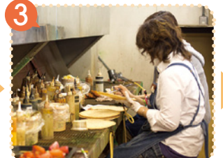
Coloring Brushes and spray paints are used to color the sample. The photo shows coloring of a pizza dough sample. Considerable experience is required to add colors for expressing the enticing aroma and texture of pizza.
