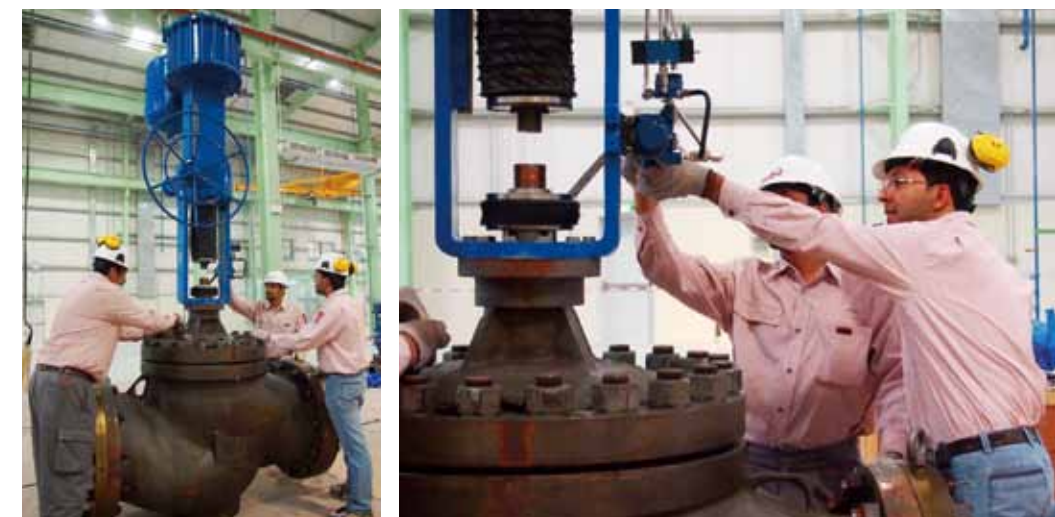
Azbil Saudi Limited employees assembling a large diameter valve.
