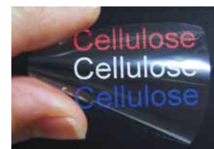
A transparent, oxygen-impermeable and durable film can be produced using cellulose nanofiber.
