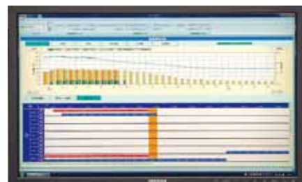
The utility optimization software package determines when to start and stop the heat source equipment by making calculations based on weather forecast data. It also shows predicted and measured temperature values, and charts of the planned and measured amounts of heat production.
