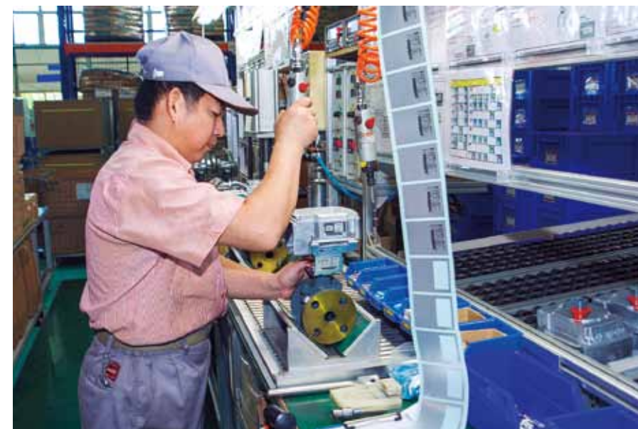
Production line for assembly of ACTIVAL™ valves for air conditioning. Valves are shipped to various countries, but mainly to Japan.
