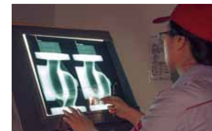
Non-destructive radiographic testing is used to check a casting for a valve.
