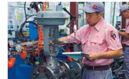
Assembled valves for industrial applications are inspected before shipment.
