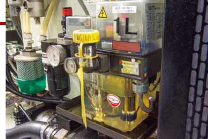
An Azbil TA's mist lubrication unit, incorporated into a machine tool, sprays lubricant on a spindle and bearing.
