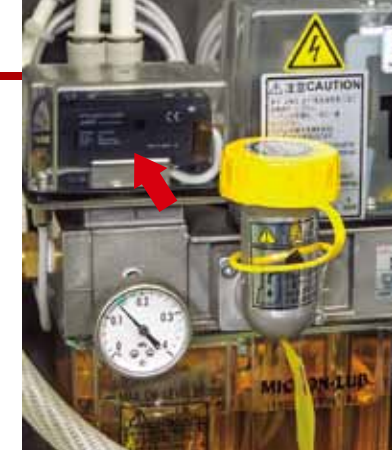
An Azbil Corporation photo-electric sensor monitors oil dropping to the venturi of Azbil TA's mist lubrication unit.
