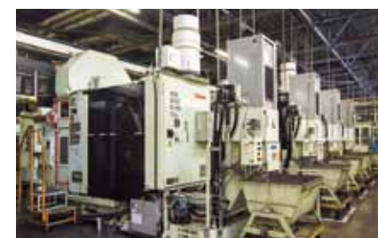
A machining center processes the head cylinder of engines at the production site at Factory 5 of the Oizumi Plant.
