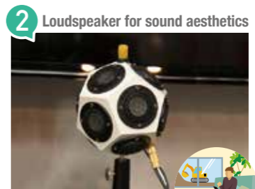
2 Loudspeaker for sound aesthetics By picking up surrounding sounds through the yellow microphone, the device analyzes the acoustics and the loudspeakers generate masking sounds to keep the auditory environment pleasant.
