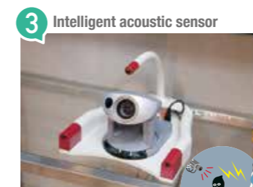
3 Intelligent acoustic sensor Analyzes and identifies the position of the sound source from signals received through multiple microphones and records the location with the camera.
