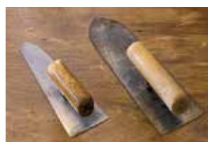
The trowel on the left has been used for more than 35 years, whereas the one on the right has been used for approximately 10 years. It can be observed that the metal sections and the handles are worn.
