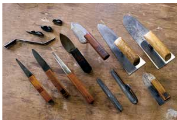
Several types of trowels are used, depending on the wall size and plaster thickness.
