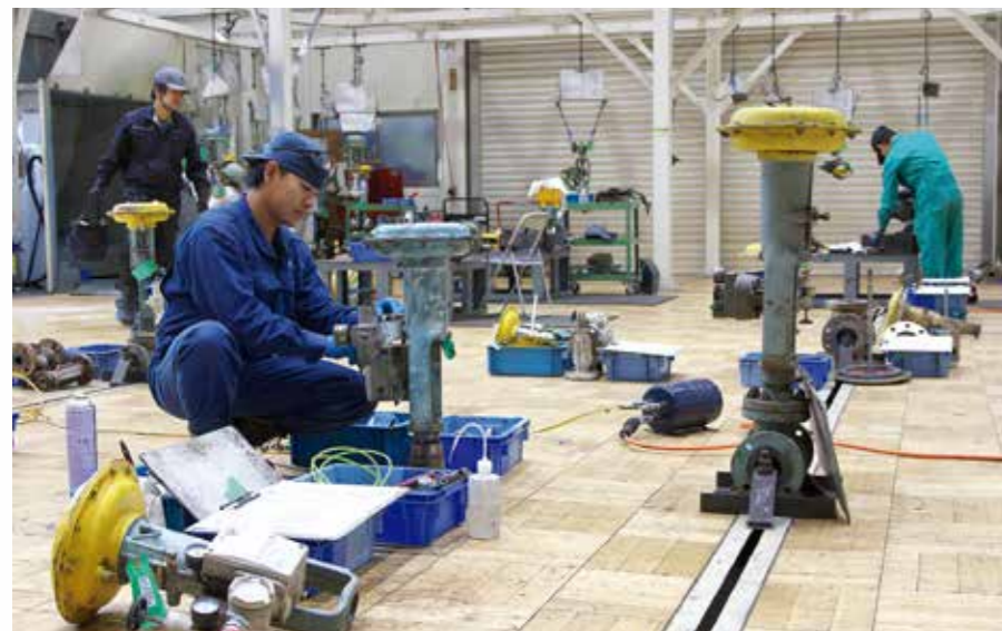
Valves are put on rails while being inspected, repaired, and maintained, in order to keep them upright. The new maintenance facility has added two more rail tracks, doubling the previous amount, and has improved its workflow to make overall maintenance performance highly efficient.
