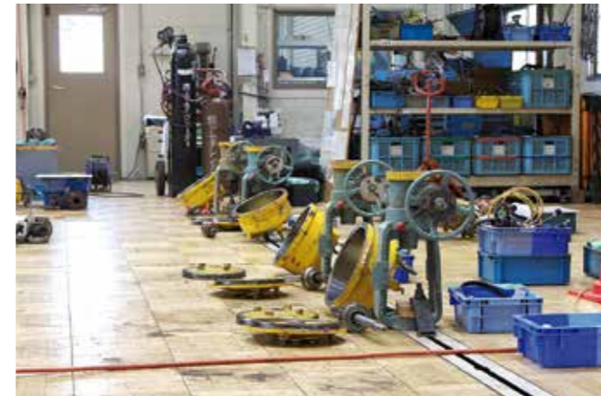
Disassembled valves from customers' plants. The inside is cleaned and, depending on the amount of wear and deterioration, valves are repaired, parts are replaced, and coating is applied. Valves are restored to like-new condition and returned to customers.
