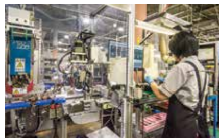
Automatic soldering machine for the sensor parts board of differential pressure / pressure transmitters. AI-based image processing judges the quality of the soldering.
