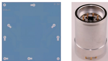
Fig. 6. Piezoresistive pressure sensor chip and package
