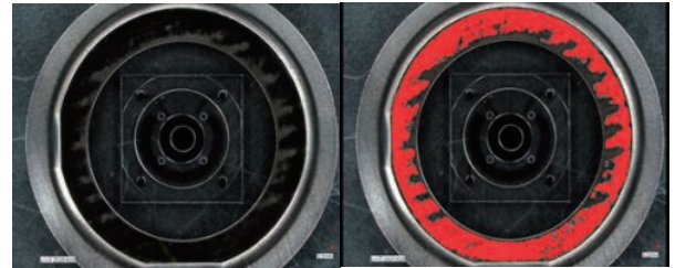
Fig. 13. Evaluation of diffusion-bonded surfaces using image processing
