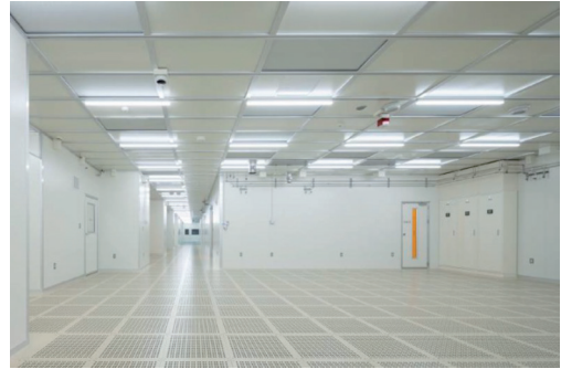
Fig. 4. Reduced number of walls in clean area
