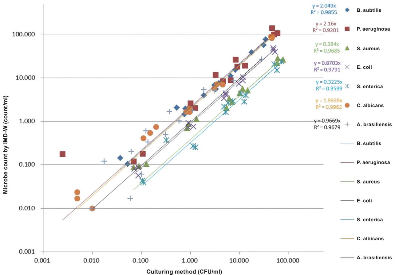
Figure 8. Scatter diagram showing microbe detection performance
