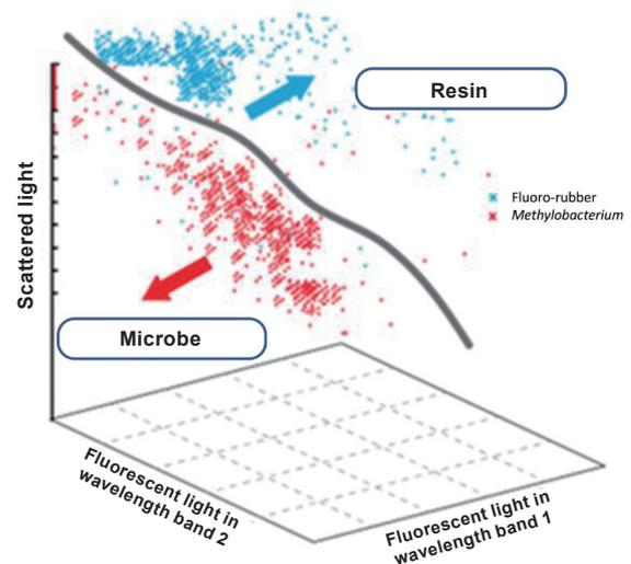
Figure 9. Microbe identification using the discrimination border
