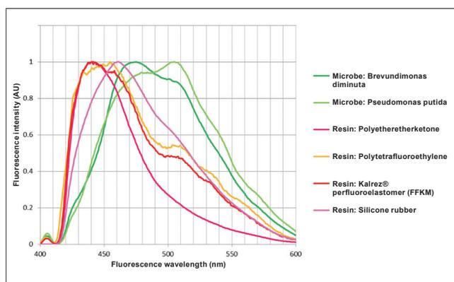
Figure 5. Fluorescence spectra from microbes and resin particles
