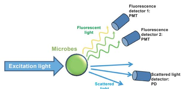
Figure 4. Schematic illustration of the optical system of the IMD-W
