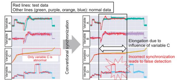
Fig. 3-3. Example of failed synchronization with the conventional method
