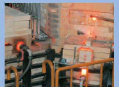
Glass making furnaces at the Otsu Plant of Nippon Electric Glass
