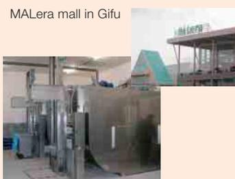
One of the largest biodegrading waste processors is installed at the MALera mall in Gifu, Japan. This system can process 750kg of garbage a day.
