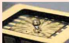
Spherical SAW sensor
