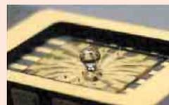
Spherical SAW sensor
