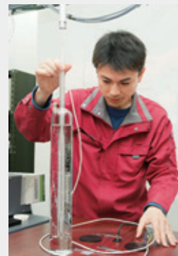
Temperature standard (Triple point of water)
