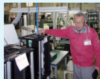
Underground water is used as cooling water in the reflow furnace
