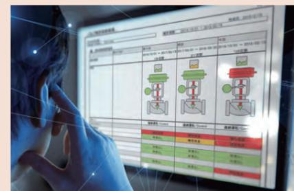
Cloud-based monitoring has enabled early detection and prediction of valve anomalies that had previously been possible only by dismantling equipment to inspect a valve’s internal condition. Cloud-based monitoring prevents trouble caused by valves and contributes to stable production equipment operation.
