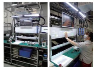
\* HCA-MS refers to a system that automates processes by mechanizing human capabilities such as the sensation of touch, eyesight, and intelligence, and combines the accuracy of machinery with the flexibility of human beings. Functionality is modular, allowing reuse and flexible response to production facility expansion or other changes.
