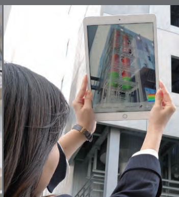
The AR shows the temperature distribution in the vertical thermal storage tanks in an easy-to-understand way.
