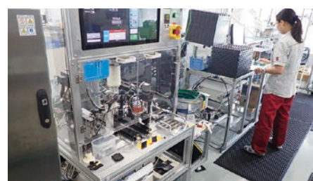
Automated assembly process for a MEMS sensor
