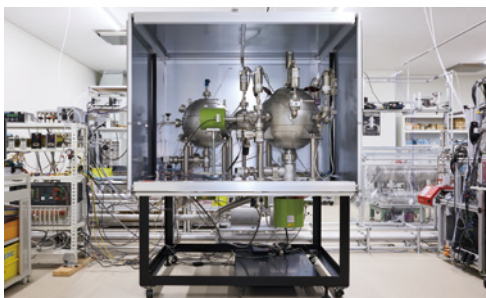
The Calibration Office at the Fujisawa Technology Center and its high-precision vacuum calibration system (center)
