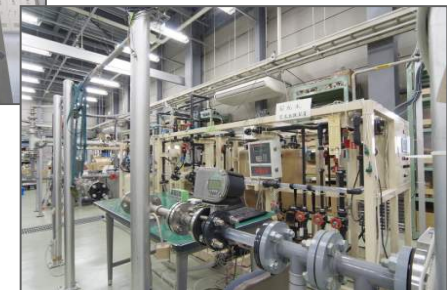
Flow Test Equipment for Development Flowmeters (Experiments can be done using a variety of fluids)
