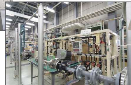
Flow Test Equipment for Development Flowmeters (Experiments can be done using a variety of fluids)
