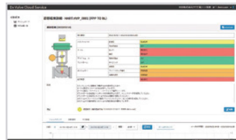
▲ Screen of the diagnosis result of the control valve maintenance support system
