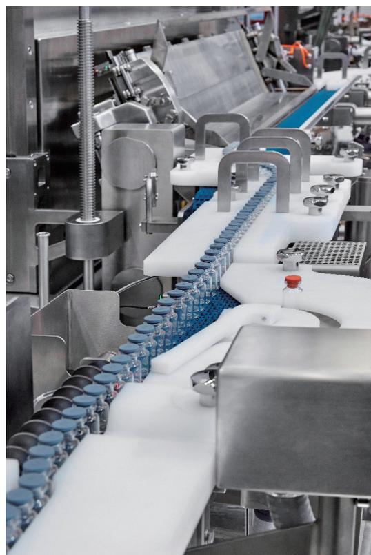
Figure 7. Vial automatic loading system
