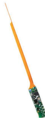
Figure 2. Sublimation interface front temperature single-use wireless probe
