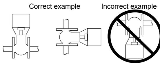
Figure 3 Installation Orientation of the Valve
