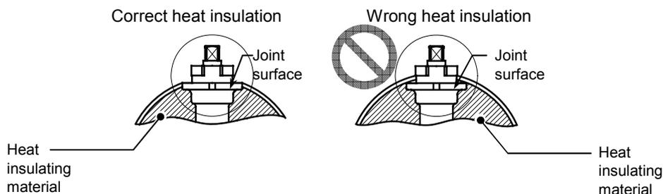
Figure 4 Heat Insulation
