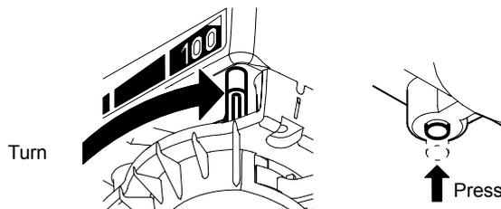
Figure 6 Indicator/Manual Lever at 100% Position (Full Open)
