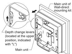
(7) Attach the main unit to the Thermoplate mounting kit.
