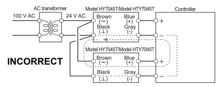
Figure 21. A loop is made in the circuit
