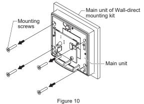
(2) Raise the main unit from the Wall-direct mounting kit. 9 mm max. can be raised.
