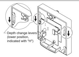
(5) Attach the main unit to the Multi-thermocase mounting kit.
