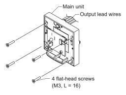
(7) Attach the cover back to the main unit. Engage the tabs (x2) located on the lower part of the cover with the slots (x2) on the lower part of the main unit. Then fix the cover with the spring, located on the top of the main unit of the sensor.
