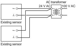
Figure 19. Wiring before replacement
