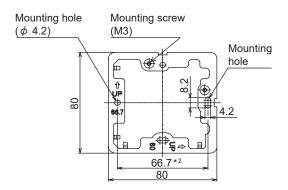
Figure 3. Surface of the mounting plate (mm)
