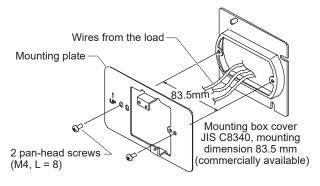
(2) Attach the Thermoplate to the mounting plate.
