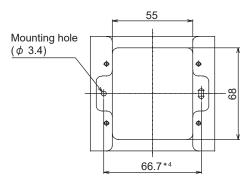
Figure 7. Surface of the Multi-thermocase mounting kit (mm)
