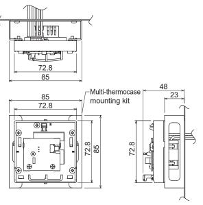
Figure 6. Dimensions when mounted in the Multi-thermocase mounting kit (mm)
