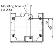
Figure 5. Surface of Thermoplate mounting kit (mm)
