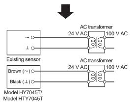
Figure 20. Wiring after replacement
