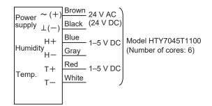
Figure 16. Wiring diagram (Room temperature/humidity sensor, 24 V AC/DC common power supply type, temperature output: 1–5 V DC type)
