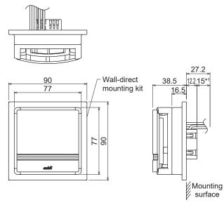
Figure 2. Dimensions when mounted on Wall-direct mounting kit (mm)
