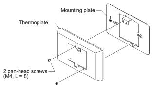
(3) Attach the main unit of the Thermoplate mounting kit to the Thermoplate.
