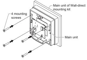
The main unit should protrude from the wall as shown in Figure 13.
