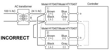
Figure 22. Incorrectly wired
