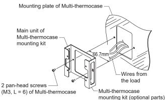
(2) Connect the lead wires of the main unit and the wires from the load.
