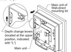
(6) Attach the main unit to the main unit of the Wall-direct mounting kit.
