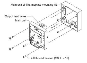
(8) Attach the cover back to the main unit. Refer to step (7) in <u>Wall-direct mounting</u>.
