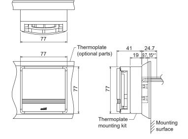
Figure 1. Main unit (mm)
