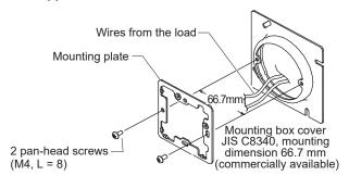
(2) Attach the main unit of the Wall-direct mounting kit to the mounting plate.
