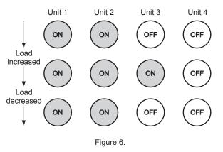
• Sequential method with base unit changeover This is one of the sequential methods.
