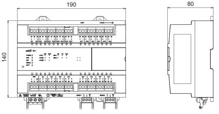
Figure 2. Dimensions (mm)
