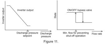
Inverter (N units) + proportional bypass valve The bypass valve and inverter are controlled by the PID control so that the discharge pressure is constant.
