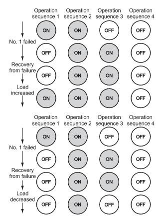
Figure 8. Operating unit precedence method (sequential)
