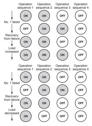
Figure 9. Sequence setting precedence method (sequential)
