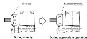
In this design, the shaft root is capped with a slitted black rubber cap. When the lever is flipped down and reaches the appropriate O.T. (overtravel), the fluorescent marking can be seen through the slit. This modification enables easy confirmation from a distance and facilitates initial setup.
