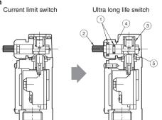
The slide-action and corrosion resistance of moving parts inside the operating head were improved.
