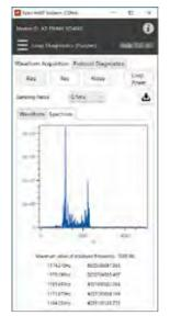
Spectrum analysis: Spectrum analysis for each frequency of communication signal can be monitored to identify the cause of noise.
