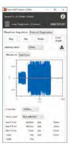
HART communication waveform can be monitored. Automatic acquisition of communication waveforms by request/response commands and the noise level can also be monitored.
