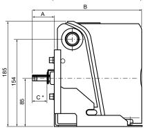
$^{\star}\,$  The C dimension shows the length of the output shaft (9.5 square).
