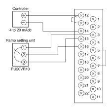
With output bias setting unit Current signal (4 to 20 mAdc)
