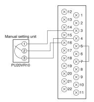
Manual setting unit and with auto / man switching Current signal (4 to 20 mAdc)
