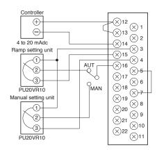
Setting unit with output indicator Current signal (4 to 20 mAdc)
