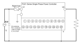
\*2 A surge generated from switch or other power circuit device may affect operation of the PU21.
