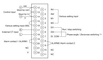
\*1 For the unit with the optional heater burnout alarm (without the display unit), the trigger of initial resistance value is set by contact input between the control input terminals (6) and (7).
