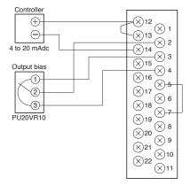
Manual setting unit, ramp setting unit with auto / Man switching
