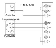
With ramp setting unit (Ramp using remote setting input)
