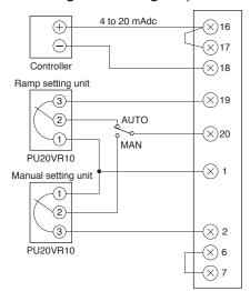
Setting unit with output indicator (Cannot be used in zero-cross control)
