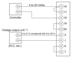
\* Output of voltage output unit needs to be insulated to connect multiple units (PU23).
