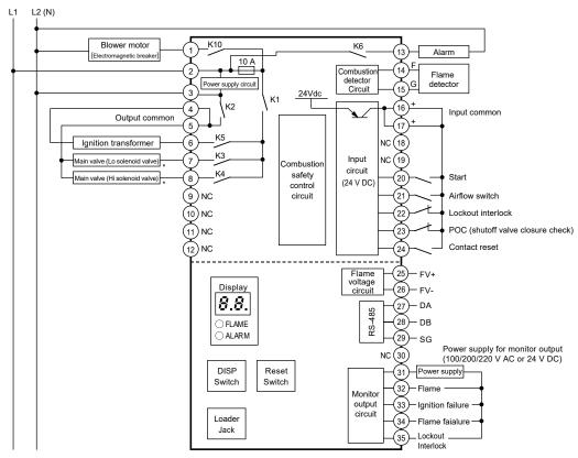
Note - Use contact reset (terminal 24) input in isolation. It cannot be used in conjunction with other BC-R contact reset inputs.
