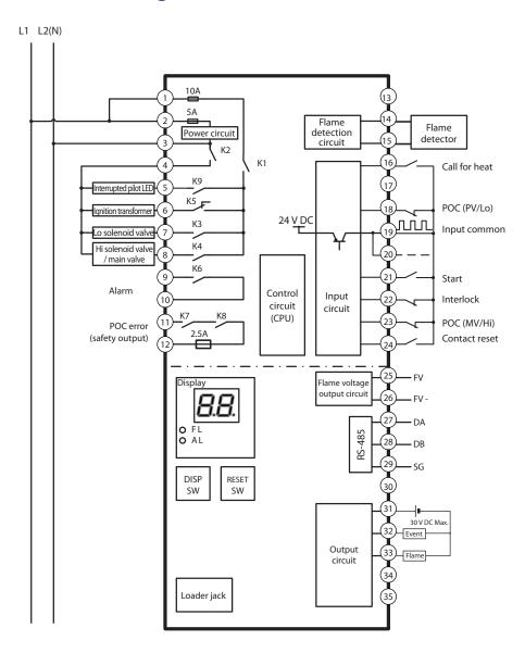
Note: • The contact reset must be used independently (by a single AUR255 device only). Do not use the terminal for contact reset of other AUR255 devices.
