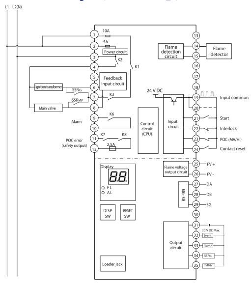
Note: • The contact reset must be used independently (by a single AUR255 device only). Do not use the terminal for contact reset of other AUR255 devices.
