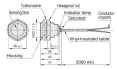
Vinyl-insulated cable (oil-resistant: 0.5 mm<sup>2</sup>, 20/0.18 dia., 2-core), dia. 5.7. Cap color: blue.
