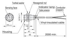
Vinyl-insulated cable (oil-resistant: 0.5  $\rm mm^2,$  20/0.18 dia., 2-core), dia. 5.7. Cap color: blue.
