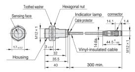
Vinyl-insulated cable (oil-resistant, vibration-resistant: 0.3 mm<sup>2</sup>, 3/20/0.08 dia., 2-core), 4.1 dia. Cap color: blue
