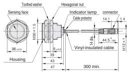
Vinyl-insulated cable (oil-resistant, vibration-resistant: 0.5 mm², 7/15/0.08 dia., 2-core), 5.7 dia. Cap color: blue
