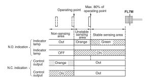
\*When the target object is made of a different material (such as aluminum, copper or stainless steel) from the standard target object (iron), the distance at which the indicator lamp changes color is shorter than the 80% maximum.
