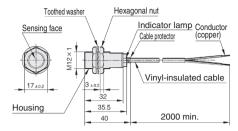
Vinyl-insulated cable (oil-resistant: 0.3  $\rm mm^2,$  27/0.12 dia., 2-core), dia. 4.1. Cap color: blue.
