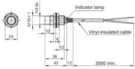
Vinyl-insulated cable (oil-resistant: 0.5  $\rm mm^2,\,45/0.12$  dia., 2-core), dia. 6. Cap color: blue.
