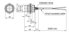
Vinyl-insulated cable (oil-resistant: 0.5  $\rm mm^2,\,45/0.12$  dia., 2-core), dia. 6. Cap color: blue.
