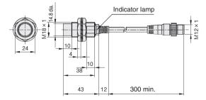
Vinyl-insulated cable (oil-resistant: 0.5  $\rm mm^2,\,45/0.12$  dia., 2-core), dia. 6. Cap color: blue.
