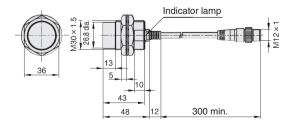
Vinyl-insulated cable (oil-resistant: 0.5  $\rm mm^2,\,45/0.12$  dia., 2-core), dia. 6. Cap color: blue.
