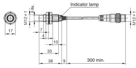
Vinyl-insulated cable (oil-resistant: 0.3 mm<sup>2</sup>, 60/0.08 dia., 2-core), dia. 4. Cap color: blue.
