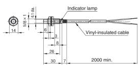
Vinyl-insulated cable (oil-resistant: 0.3 mm<sup>2</sup>, 60/0.08 dia., 2-core), dia. 4. Cap color: blue.
