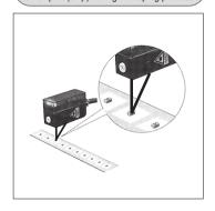
Detecting the presence/absence of a wafer disk based on the disk edge
