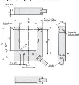
\*Cable specifications: oil-proof, O.D. 4.2 mm, 3-core, nominal cross-sectional area 0.2 mm², sheath color gray.
