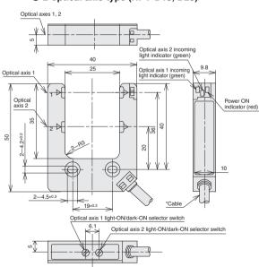
\*Cable specifications: oil-proof, O.D. 4.2 mm, 4-core, nominal cross-sectional area 0.2 mm², sheath color gray.
